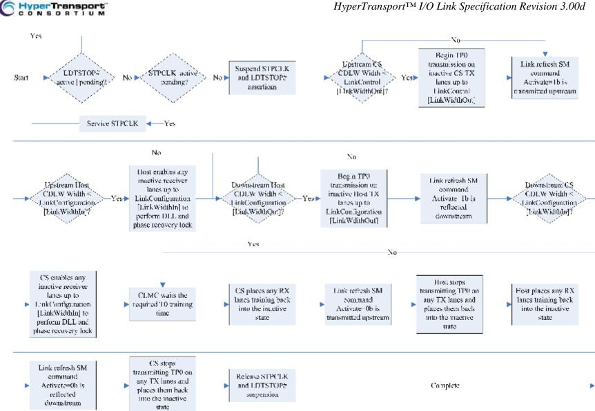
Figure 12. CLMC Sequencing Diagram for CILR
