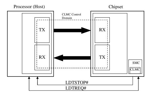
Figure 10. Centralized Link Power Management Control Topology
