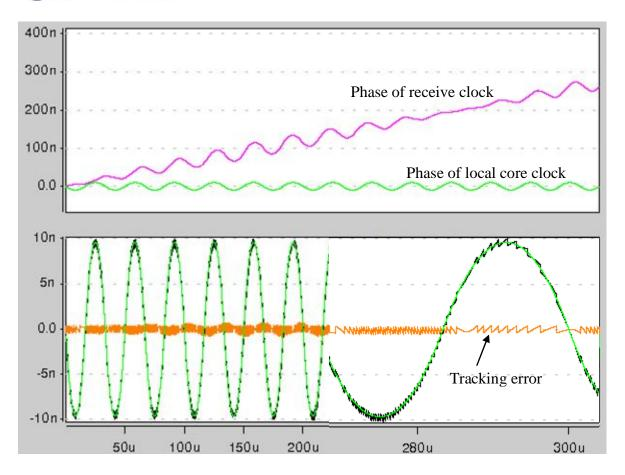
Figure 65. Phase tracking across receiver sync-fifo
