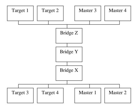
Figure 26. Example PCI System
