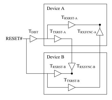
$T_{RXRST}$  – The delay from assertion of RESET# at the device pin to when inputs are ignored at an internal state commit point. <T<sub>RXSYNC</sub> recommended.
