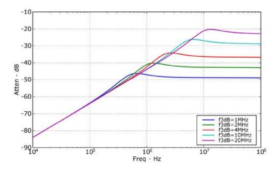
Figure 49. System reference clock jitter rejection
