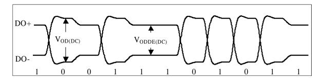
Figure 33.  $V_{ODDE(DC)}$
