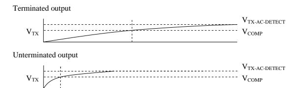
Figure 19. AC Detect Timing
