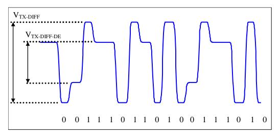
Figure 51. Differential transmitter post-cursor de-emphasized waveform
