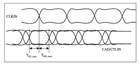
Figure 46.  $T_{SU}$  and  $T_{HD}$
