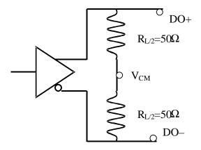
Figure 31. DC Output Reference System Load
