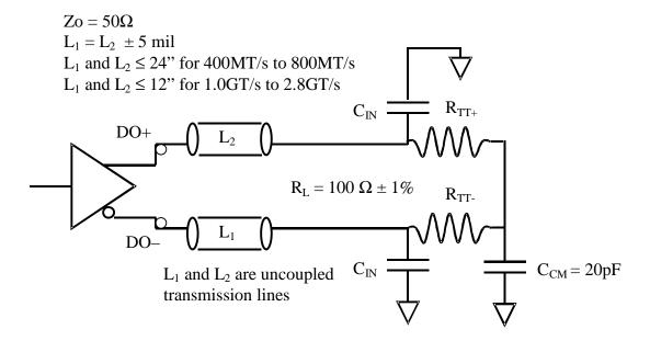
Figure 37. AC Reference System Load (See Table 167 for C<sub>IN</sub>, R<sub>TT+</sub> and R<sub>TT</sub>)
