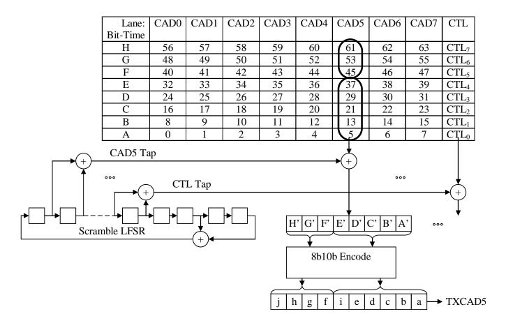
Figure 4. Gen3 Transmitter Order of Operations
