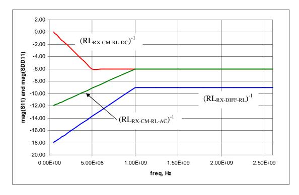
Figure 58. Receiver return loss mask
