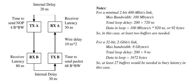
Figure 8. Example Gen1 Data Buffer Sizing Calculation
