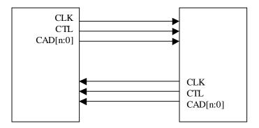
Figure 1. HyperTransport<sup>TM</sup> I/O Link
