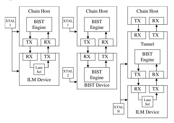
Figure 22. Link Test Topologies
