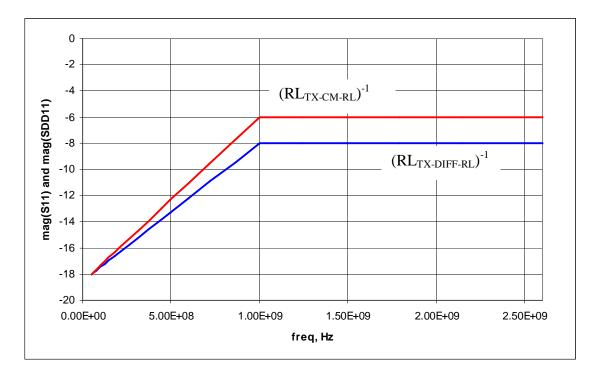
Figure 50. Transmit return loss mask
