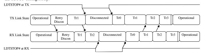
Figure 20. Example LDTSTOP Disconnect Sequences
