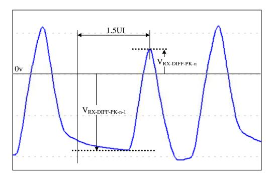
Figure 61. Receiver adjacent bit ratio
