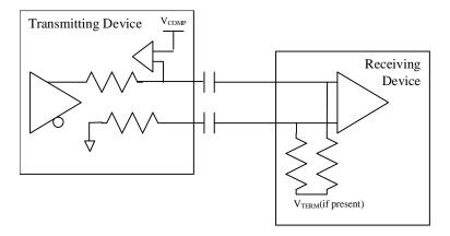
Figure 18. AC Detect Circuit
