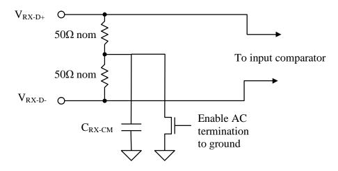
Figure 59. Receiver input termination
