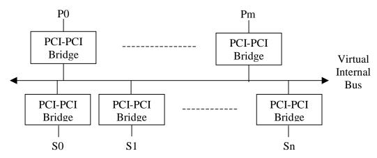
Figure 29. Logical Model of a Switch
