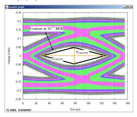
Figure 57. Channel compliance eye diagram
