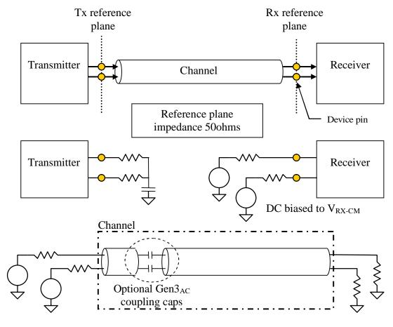
Figure 48. Measurement methodology of HyperTransport  $^{TM}$  link components
